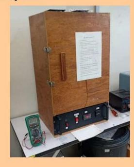
Temperature is increasing but always below 75 °C for the time/round of 10 mins. UV Dose =  $120 \text{ mJ/cm}^2$
